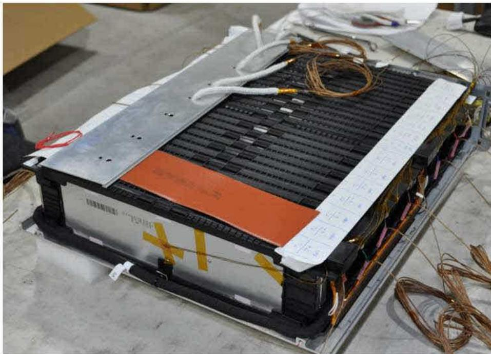
Figure 28 Photograph showing the thermocouple attached to the outer surface of the Cell 7 pair.
