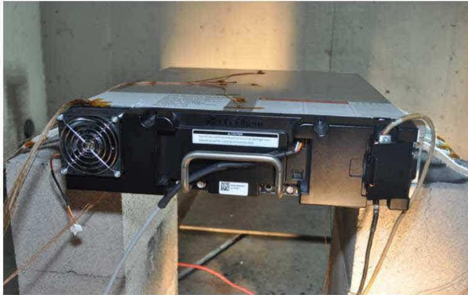
Figure 32 Photograph showing the front face of the module pre-test, with the communication cable and charging cables attached.
