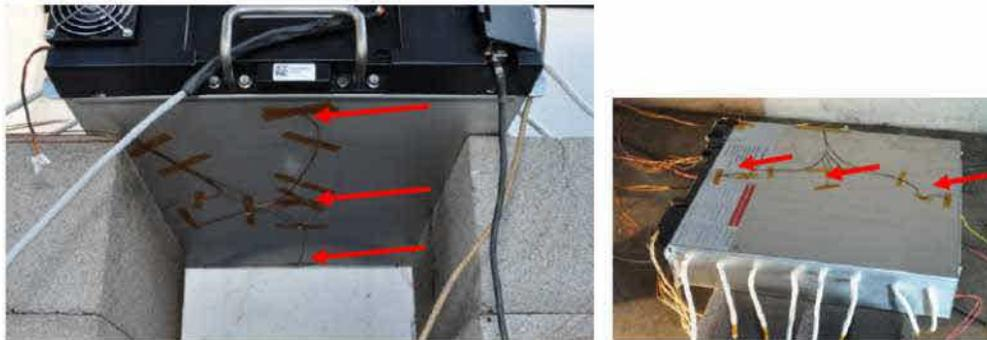
Figure 30 Photographs showing three thermocouples attached to the bottom (left) and top (right) panels of the module along the centerline in the front, middle, and rear.
