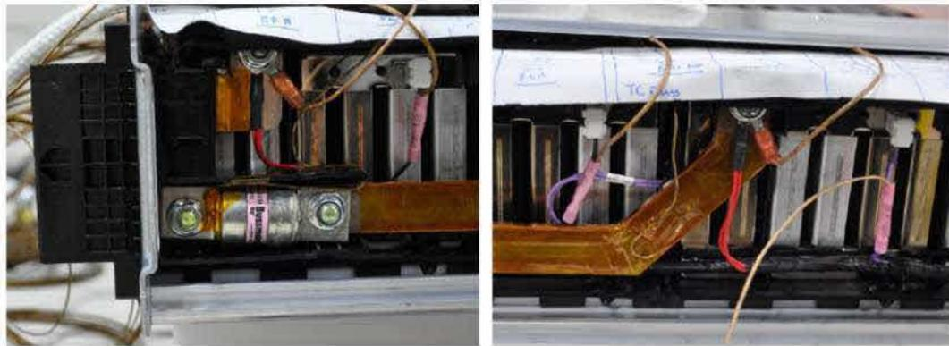
Figure 29 Photograph showing thermocouples attached to the negative busbar fuse (left) and busbar (right).
