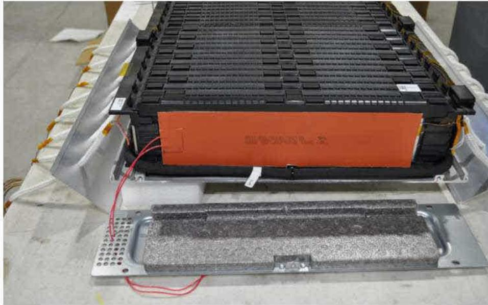
Figure 31 Photograph showing the heated pad installed on outer surface of the Cell 7 pair.
