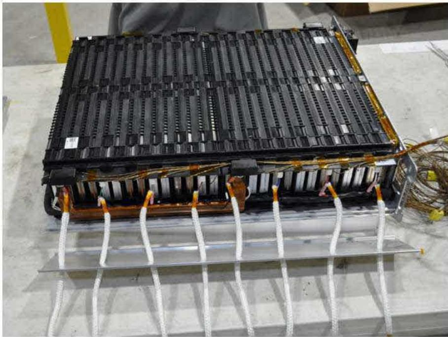
Figure 27 Photograph showing the installation of voltage taps and cell thermocouples.
