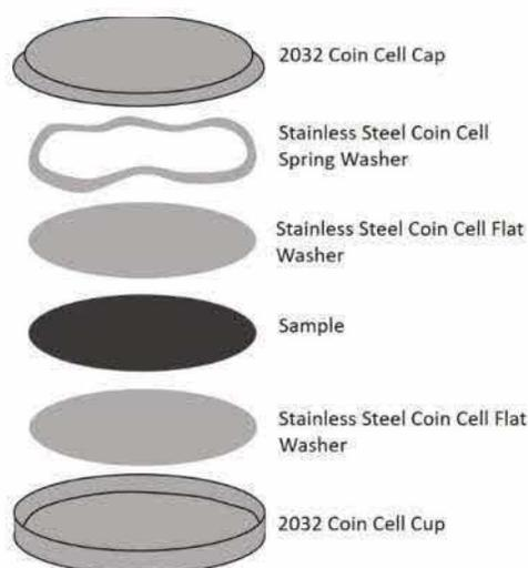
Figure 74 Schematic of the experimental setup for conductivity testing of negative electrode materials.
