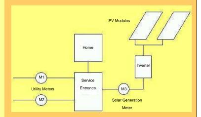
The electricity generated by your solar system (M3) can only go to two places – EITHER into your home to feed electrical loads running in your home OR into the utility power grid.
